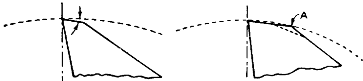
Figure 13.-Width of land increases with repeated sharpenings, causing interference at A. Grind clearance angle as shown by dotted line to control width of land.
